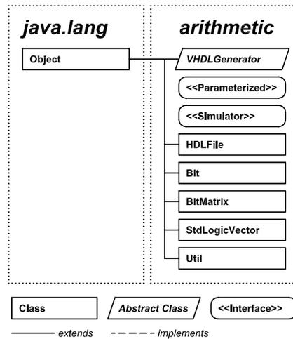
Fig. 4. The arithmetic package
